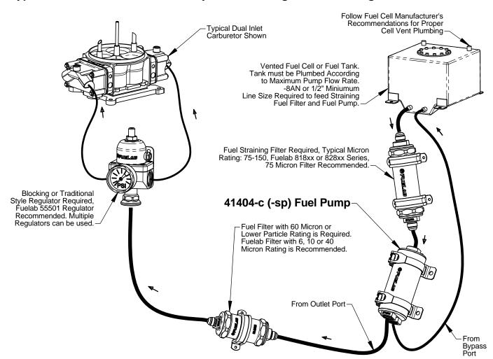
Special Note: This model of pump incorporates an external bypass valve, and therefore is capable of being "dead-headed".
